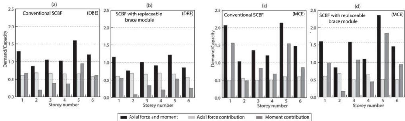
Figure 5. Median demand-to-capacity ratios of columns in SCBF columns: (a)conventional SCBF (DBE), (b)SCBF with replaceable brace modules (DBE) (c)conventional SCBF (MCE), (d)SCBF with replaceable brace modules (MCE)
