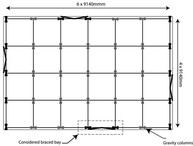
Figure 2. Plan configuration of 6-storey building
