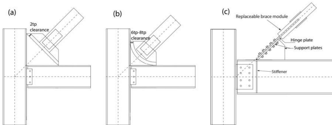
Figure 1. Brace to frame elements connection details: a) Typical gusset plate with linear hinge zone b) Typical gusset plate with elliptical hinge zone c) New proposed connection with replaceable brace module
