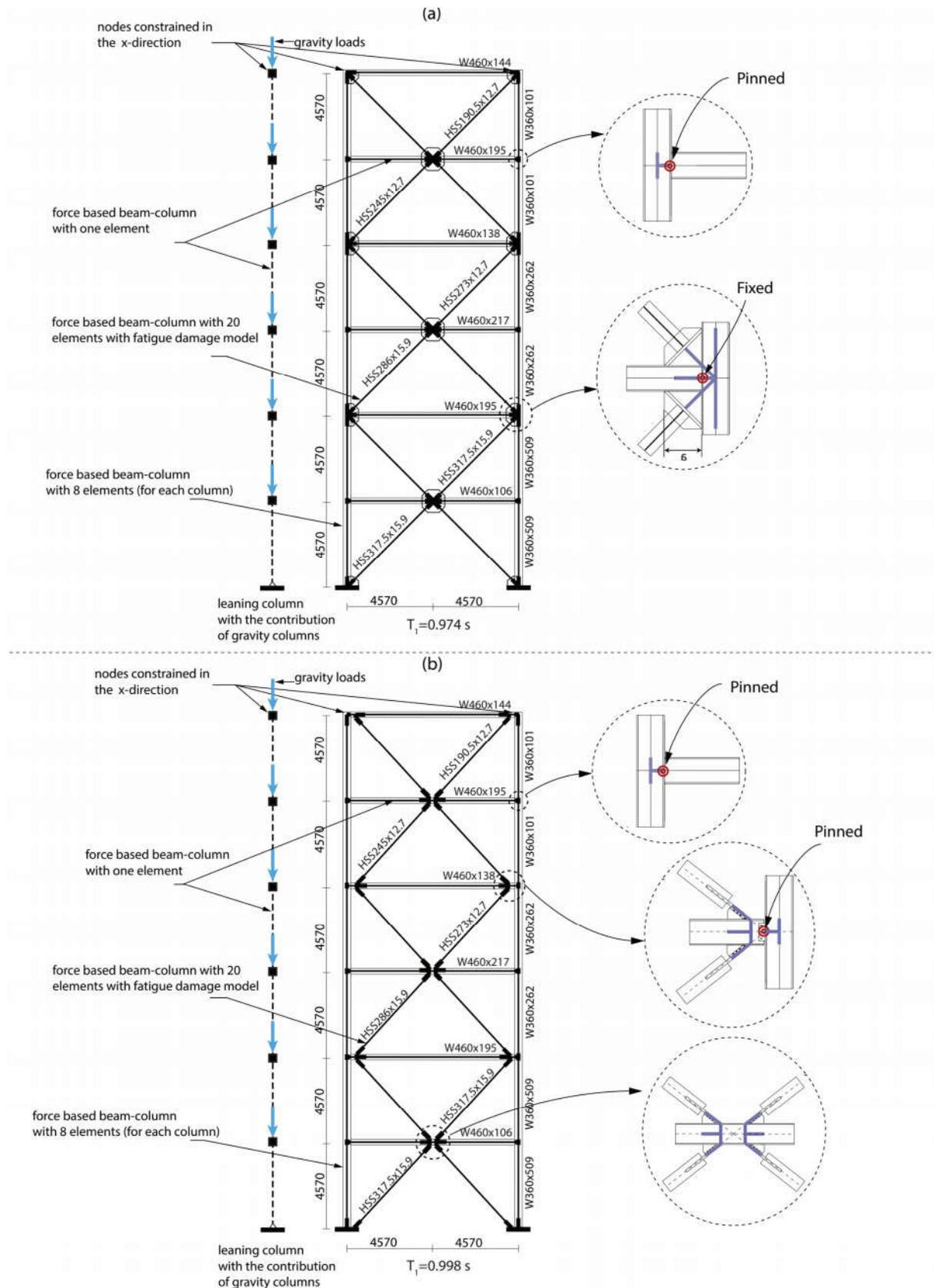
Figure 3. a) Schematic of the numerical model for six-storey SCBF with conventional connection. b) Schematic of the numerical model for six-storey SCBF with replaceable brace modules
