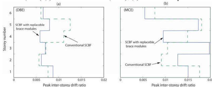
Figure 6. Median inter-storey drift ratio: (a)DBE and (b)MCE
